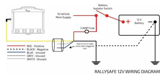
During installation, the wiring loom should be routed away from the engine compartment, Ignition or Alternator wiring.
